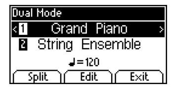
At this step the the "F1" button allow to cycle through Dual, Split or 4-Hand mode
